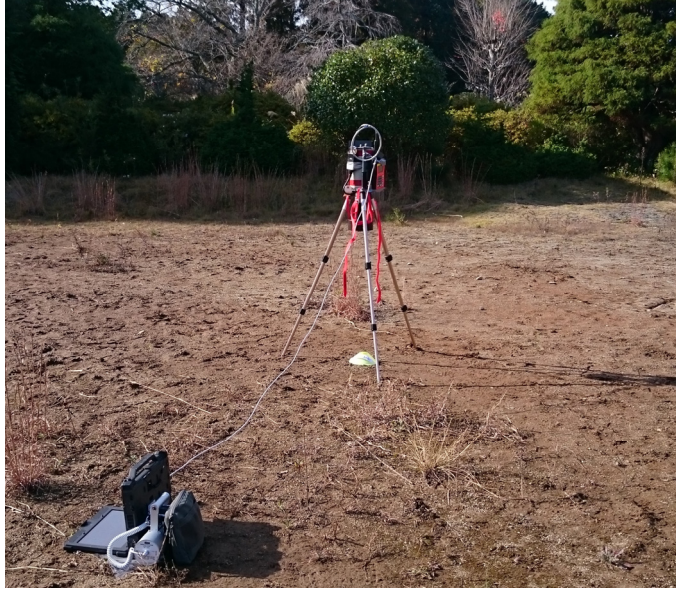
Figure 12. Typical measurement geometry in Fukushima prefecture outside the Fukushima Daiichi nuclear power station in 2015, where measurements were performed at a sports field with as flat a ground surface as possible within the field of view of the detector. The collimator was applied to the detector and is visible hanging in the red straps.
