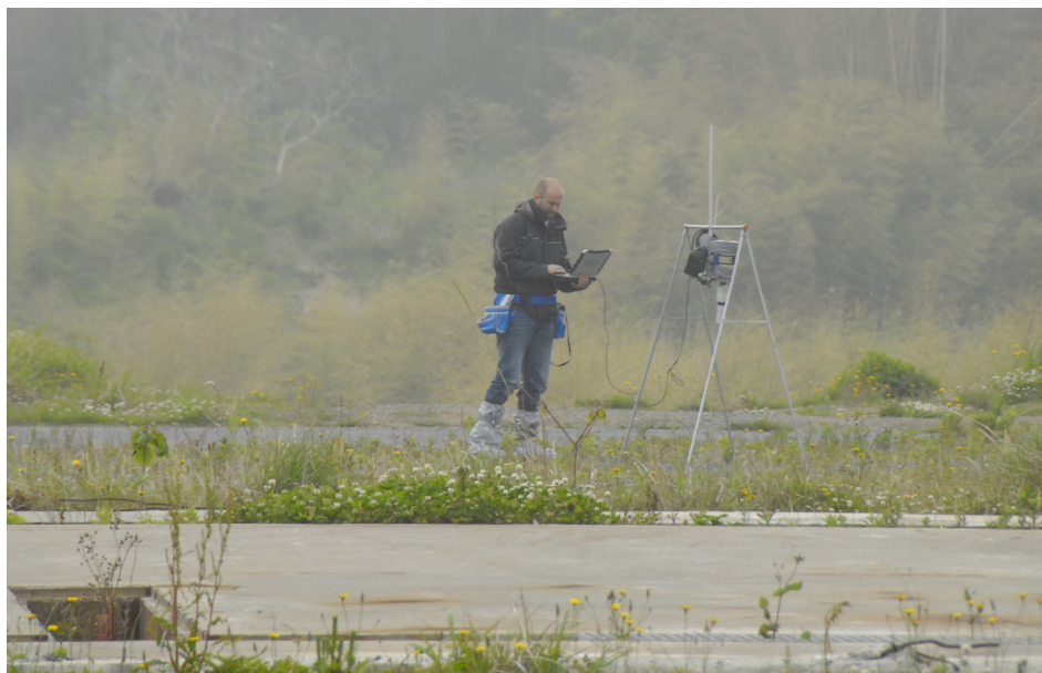
Figure 5. PTV measurements close to the fence of the Fukushima Daiichi reactor site in 2013 using a thin steel frame to cause minimal obstruction of the ^{134}, ^{137}\text{Cs} photon field.
