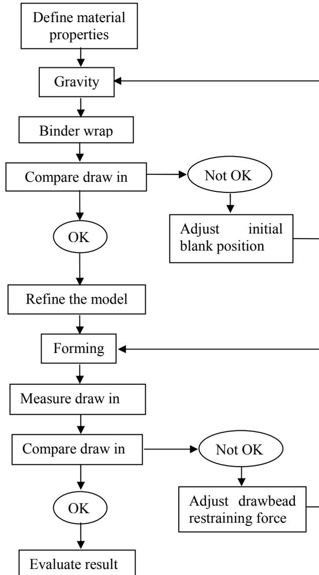
**Figure 7:** Flow chart of the simulation procedure.
