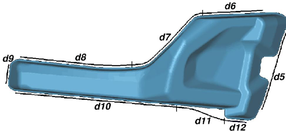
*Figure 9: Equivalent drawbead locations in the FE model.*
