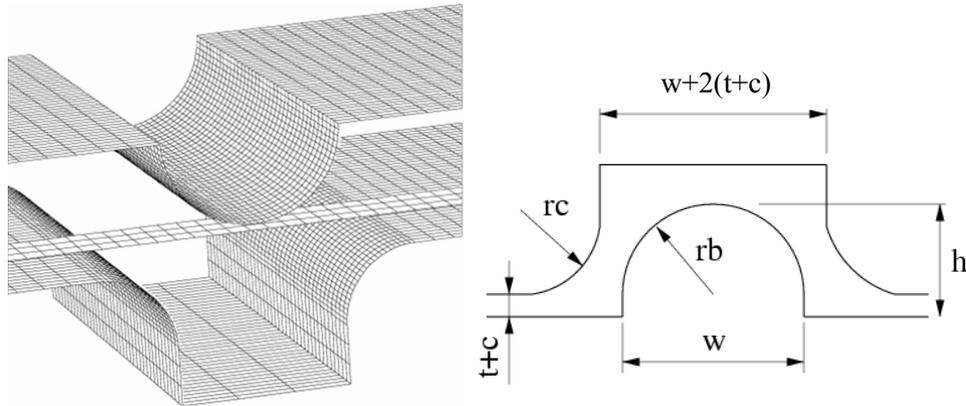
**Figure 12:** Simulation lay-up and parameters in the drawbead.
