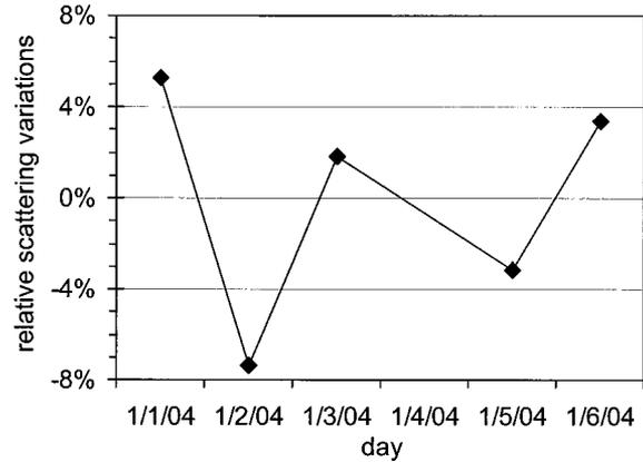
Fig. 7. Reproducibility plot for  $\mu_a$  obtained on phantom  $T_a$ , using instrument 7 at 780 nm, in a reflectance geometry, with  $\rho = 1$  cm. The plot represents the relative displacement of  $\mu_{a, \text{meas}}$  obtained at each measurement day with respect to the average value calculated over 5 days.
