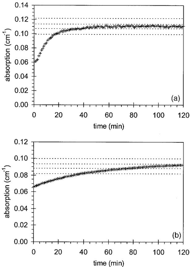
Fig. 6. Stability plot for  $\mu_a$  obtained on the phantom  $T_a$ , using (a) instrument 8 at 690 nm, in a reflectance geometry, with  $\rho = 2$  cm and (b) instrument 4 at 785 nm, in a transmittance geometry. The dashed lines correspond to  $\pm 3\%$  and  $\pm 10\%$  changes with respect to the average of  $\mu_a$  over the last 30 min of measurement.
