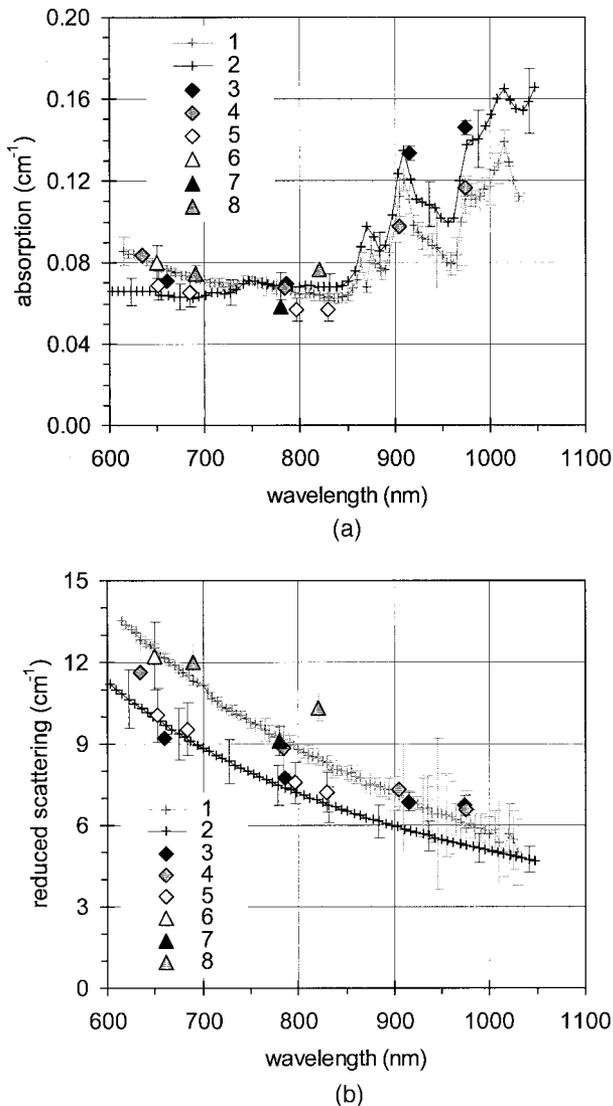
Fig. 2. Comparison of the estimate of (a)  $\mu_a$  and (b)  $\mu_s'$  obtained by the eight instruments on the phantom B2. The measurements are performed in transmittance geometry for instruments 4, 5, and 6; in reflectance geometry with  $\rho = 2$  cm for instruments 1, 3, 7, and 8; and in reflectance geometry with  $\rho$  variable in the interval 0.2–1.8 cm in steps of 0.2 cm for instrument 2.
