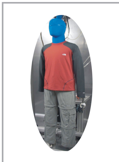
Figure 2. Fabric sweating thermal manikin “Walter”.
