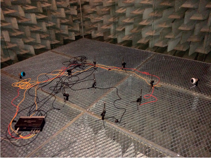
Figure 7: A photo showing the experimental setup in the anechoic chamber, where eight sensors are used to record two coherent sources.
