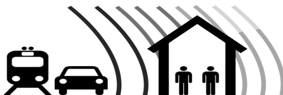
Figure 1. The concept of quiet side, a sheltered side of a dwelling where noise levels are lower than at the most exposed side.
