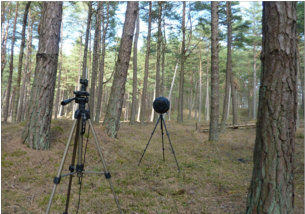
Picture 3. Measuring impulse response in pine forest.
