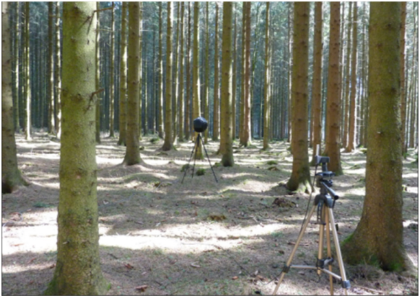
Picture 4. Measuring impulse response in fir forest.
