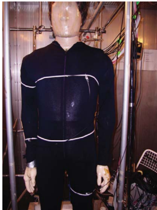
Fig. 1. The thermal manikin 'Tore' in the climatic chamber.
