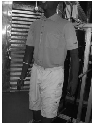
Fig.1.3 Sweating thermal manikin at INAIL, Italy (Newton, MTNW, Seattle, WA)
