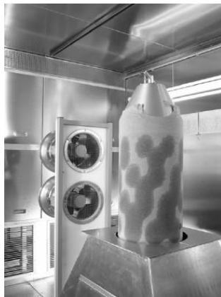
Fig.1.2 Sweating torso at EMPA, Switzerland (©Keiser 2007)
