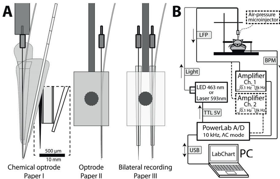
**Figure 5. Optrodes and *in vivo* recording setup**
