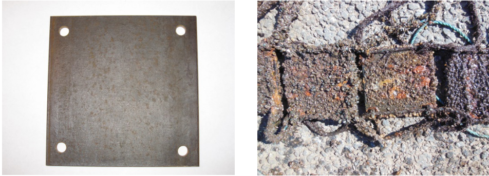
Figure 41 Steel plates before and after exposure.
