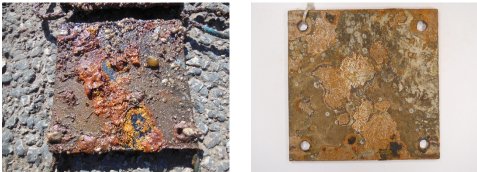
Figure 42 Steel plate before and after cleaning.
