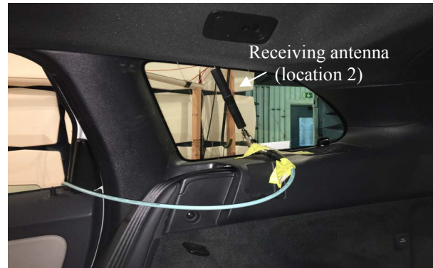
Fig. 2. Receiving antenna at the rear right quarter glass (receiving location 2).
