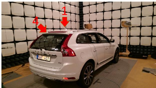
Fig. 2. The Volvo XC60 and the positions of two receiving antennas used in the measurement.
