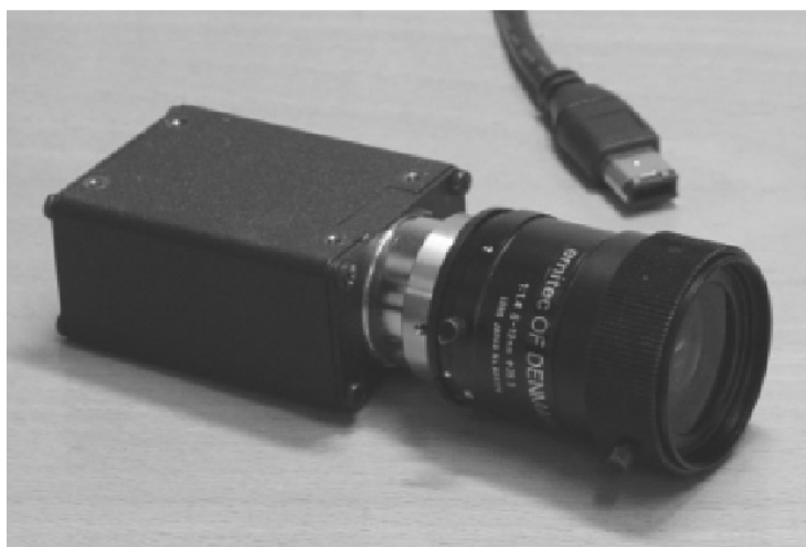
Figure 2.2 Firewire camera Basler A602fc and standard 6-pin connector.
