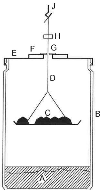
Figure 1. Drawing of the jar used in the measurements of sorption isotherms. A: saturated salt solution; B: glass jar; C: material to be investigated; D: wire; E: lid; F: metal plate; G: transparent washer; H: stop; J: hook on balance for under-weighing.
