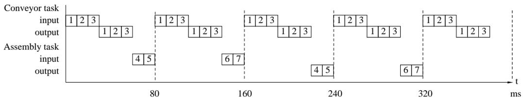
But when this system was implemented and run, we found that the system occasionally did misfeed cars. Logging of the activity revealed that the RS-232 bus was allocated as follows:
