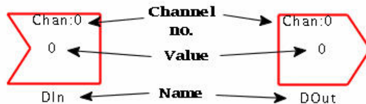
Figure 3.24 Digital input (left) and output (right).
