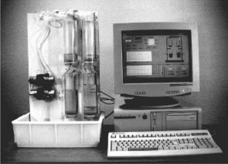
**Figure 1.** The quadruple-tank laboratory process shown together with a new controller interface running on a Pentium PC.
