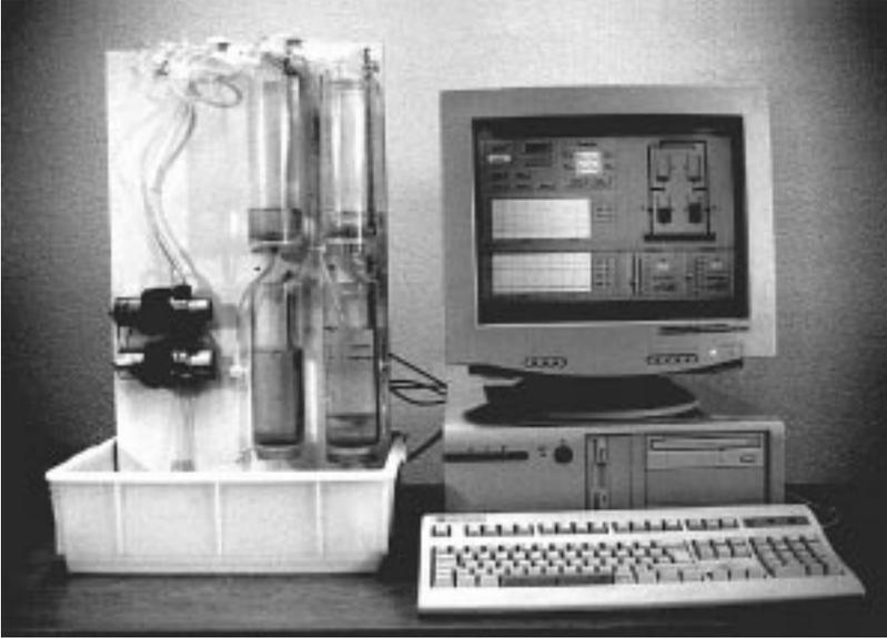
**Figure 1.** The quadruple-tank laboratory process. The water levels in the lower two tanks are controlled with the help of two pumps.
