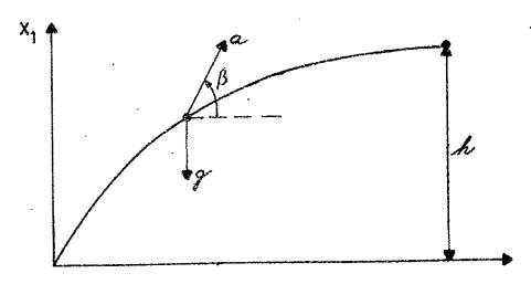
Study the motion of a rocket in a constant gravitational field. The thrust has a constant magnitude a, but the thrust angle  $\beta$  is a control variable. If  $x_2$  denotes the vertical component of the velocity, the equations of motion are
