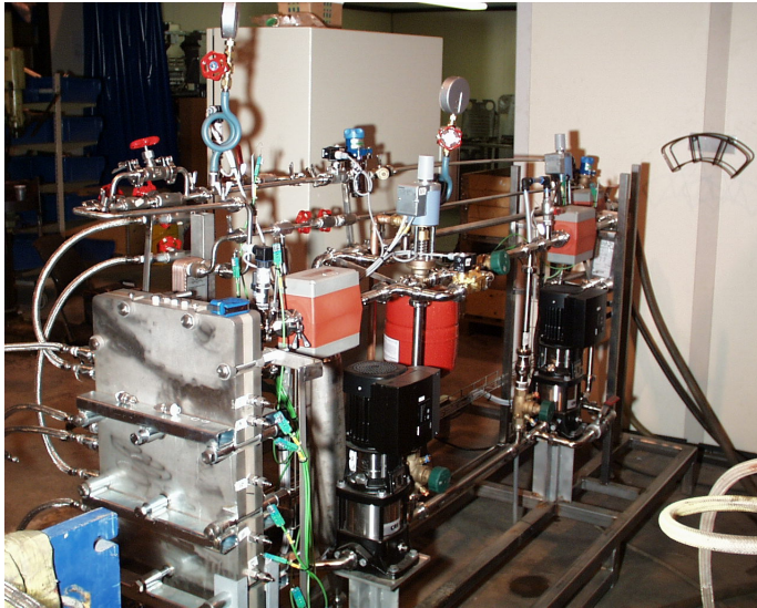
Figure 5.11 The experimental test unit, with the plate reactor to the left.
