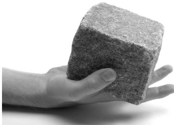
FIGURE 1. A small paving stone (Sw. smågatsten ) from the streets of Lund. 8 x 8 x 10 cm. Weight 2.2 kg. Photo: B. Almgren, Historical Museum, Lund University.
