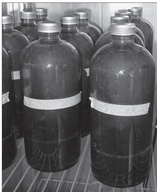
Figure 1. Reactors for determination of methane potential (2-litres glass bottles with septum corks).
