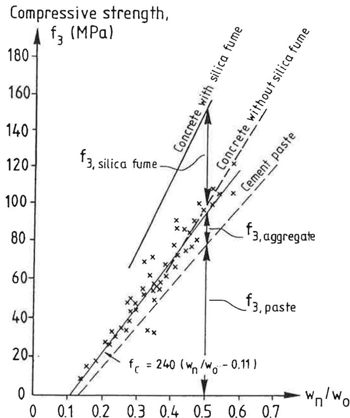
Figure 6 Compressive strength,  $f_3$ , as function of hydration factor,  $w_n/w_0$ . (— = 10% silica fume of the cement content, - - - = concrete without silica fume, x—x = cube results acc to **Powers (1948)** for cement paste; - - - = recalculated to cylinders).
