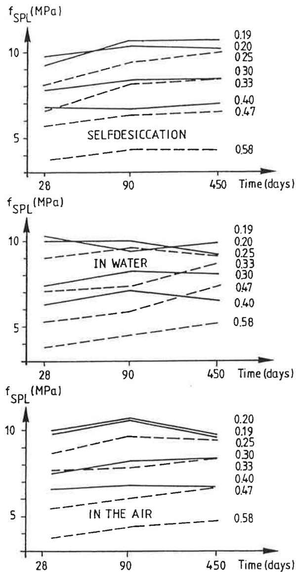
Figure 4 Split tensile strength,  $f_{spl}$ , as function of time.
