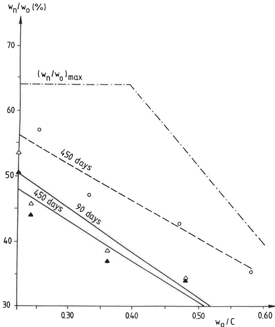
Figure 5. Hydration factor,  $w_n/w_o$ , as function of water-cement ratio. Figures indicate number of mixture. (— = 10% silica fume, --- = no silica fume).
