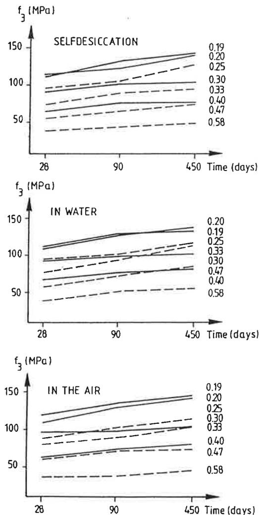
Figure 2 Compressive strength,  $f_3$ , as function of time.
