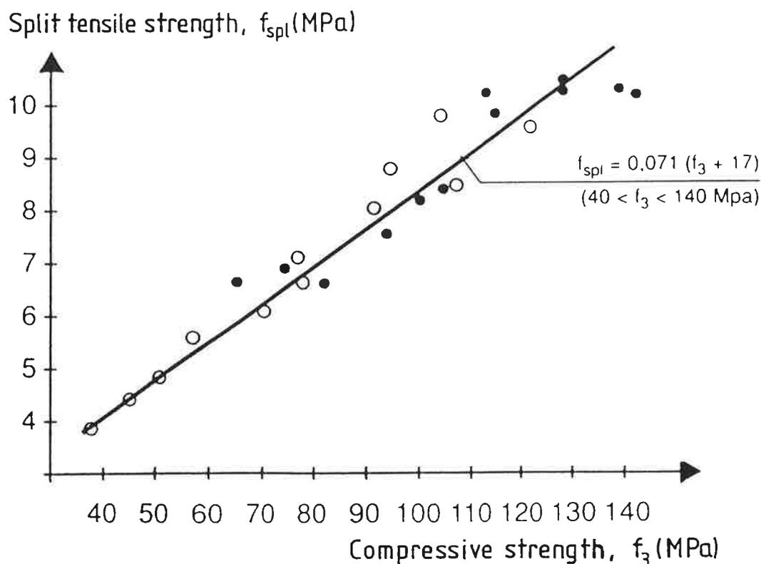
Figure 3. Split tensile strength,  $f_{spl}$ , related to compressive strength,  $f_3$ . (• = 10% silica fume of the cement content, o = no silica fume).
