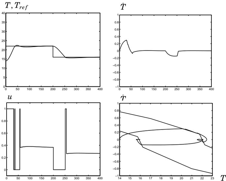
**Figure 5.11** Simulation of the ventilation model for the school in Klippan. The affine approximation of the ideal switching curves is seen together with two set-point change trajectories in the last sub-plot.
