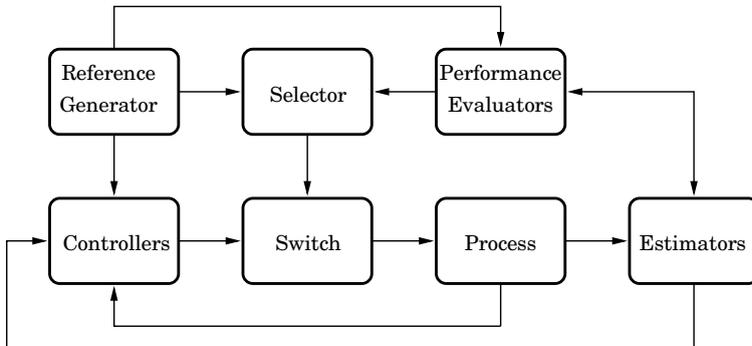
**Figure 1.2** A block model of a general hybrid control system.
