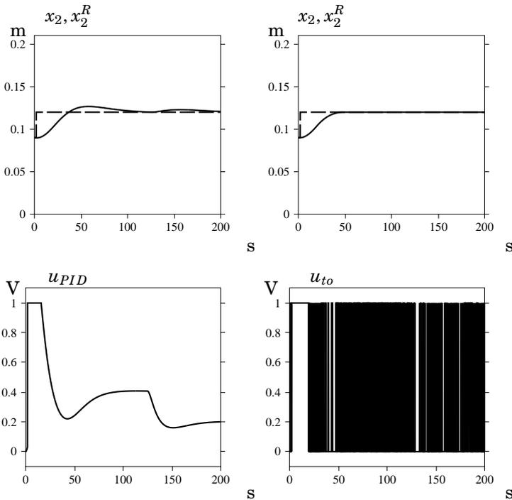
**Figure 5.3** Pure PID (left) and pure time-optimal control (right). The PID controller has a smooth control signal but gives a slow response with an overshoot. The time-optimal controller gives a fast response but the control signal is unusable in practice
