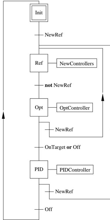
**Figure 5.2** A Grafcet diagram describing the control algorithm.
