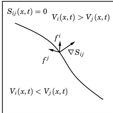
**Figure 4.3** The figure shows a phase plane close to the switching surface  $S_{ij}(x, t) = V_i(x, t) - V_j(x, t) = 0$ . The control law corresponding to the smallest Lyapunov function is used. Under certain conditions, see Equation 4.9, there will be a sliding motion on the switching surface.
