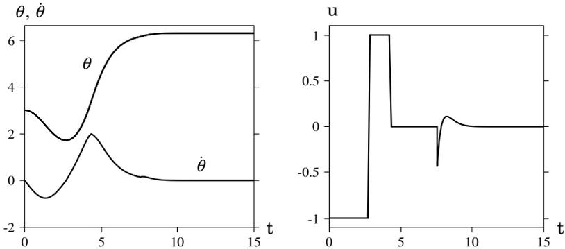
**Figure 4.7** Simulation of the pendulum using the switching strategy based on  $\min(V_E, V_{FB})$ . Only one switch occurs, at time  $t = 7.34$ , from the control law  $u_E$  to  $u_{FB}$ . The system is caught and stabilized in the upright position.
