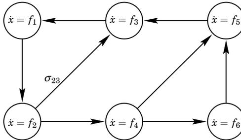
**Figure 1.7** Graph of a Tavernini-type hybrid system.
