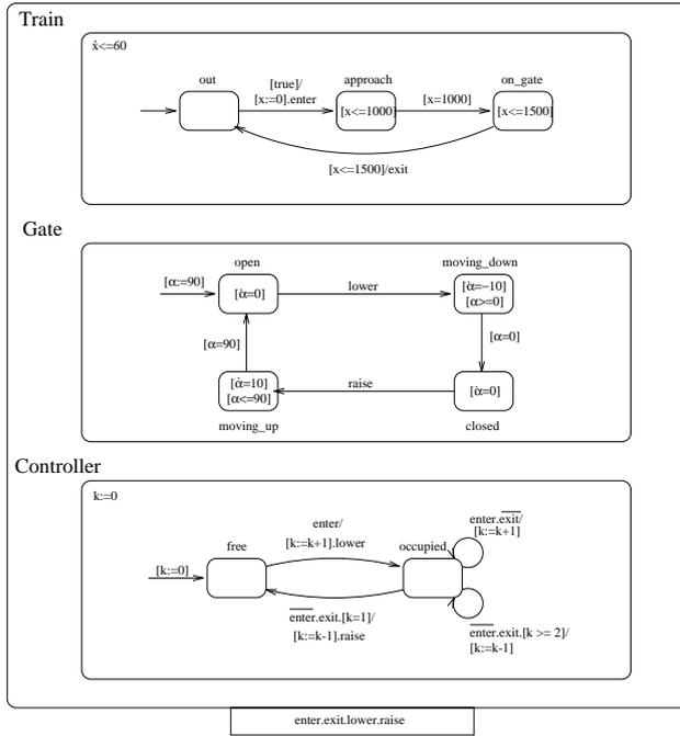
Figure 1.10 Three automata, one for each subsystem.
