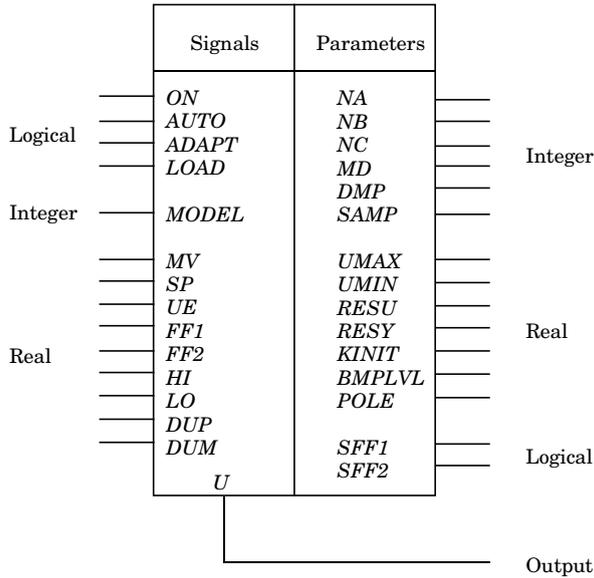
**Figure 1.5** The expert module STREGX in Firstloop. Picture taken from Åström and Wittenmark (1995) p. 513.
