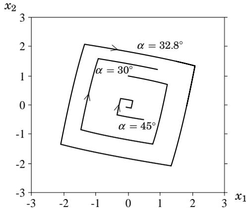
**Figure 4.4** Simulation of Example 4.3 with  $\alpha$ -strategies. The stability of the ad-hoc switching strategy depends on  $\alpha$ . The switching strategy defined by the Lyapunov functions in Equation 4.11 corresponds to  $\alpha = 45^\circ$ , which gives a stable system.
