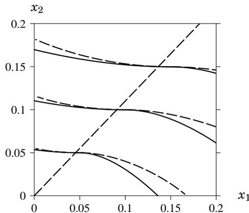
**Figure 5.4** Linear (full) and nonlinear (dashed) switching curves for different set-points. Above the switching lines the minimum control signal is applied. Below the lines the maximum control signal is used
