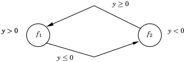
**Figure 2.2** The hybrid automaton for Example 2.1.
