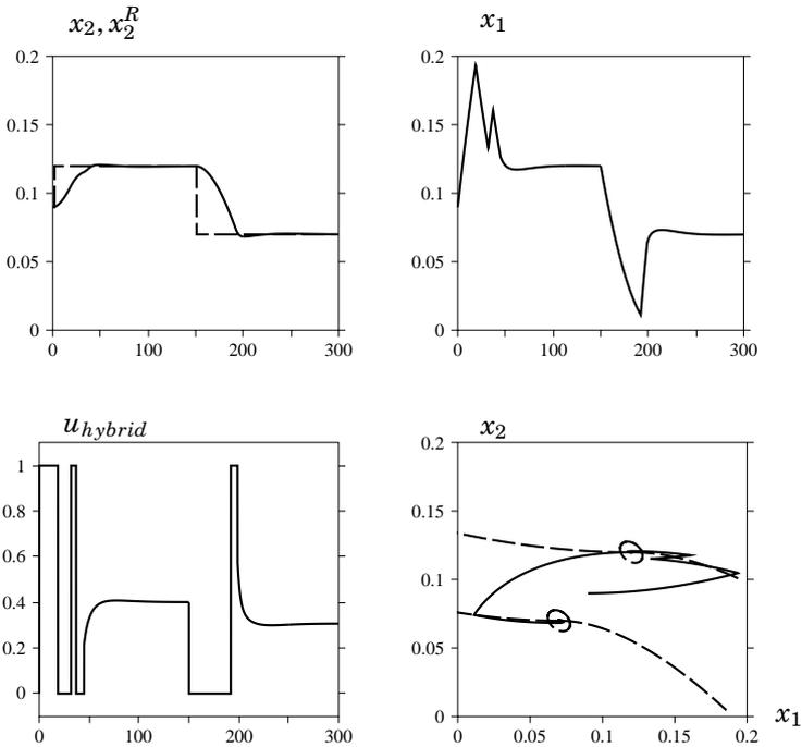
**Figure 5.5** Simulation of the simple switching strategy. Lower left figure shows the control signal. The time-optimal controller makes one extra min-max switch because of the nonlinearity. Catching regions are shown in lower right sub-figure.
