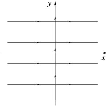
**Figure 3.1** Phase plane for Example 3.3. The vectorfield is vertical for  $x = 0$  and horizontal for  $x \neq 0$ . The solution  $x \equiv 0, y = 1$  is not considered a solution according to definition 2.
