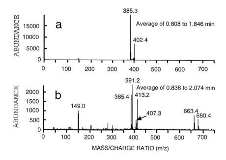
Fig. 2. ESI-MS analyses of authentic vitamin D (a) and *C. arbuscula* sample (b). Peaks at m/z 385.3 and m/z 402.4 represent  $[M-H]^+$  and  $[M-NH]_4^+$ , respectively. The peak at m/z 385.4 shows that the sample contains vitamin D<sub>3</sub>.
