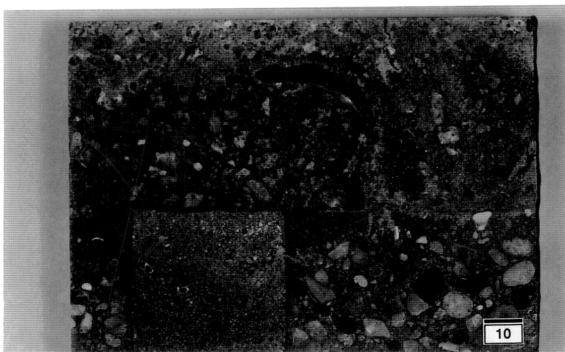
Photo 6. Microstructure and chloride penetration in concrete corrosion cell. Slag cement w/c ratio 0.40, after 8 months exposed to cycles of 2 hours wetting in a 16 % NaCl solution and 166 hours drying in the laboratory at room temperature. Electrode without filter paper defect.
