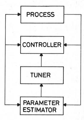
Fig. 5.1. Structure of control loop with on-line tuning.
