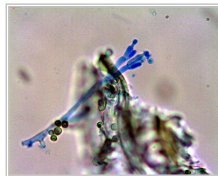
Figure 7.2 Microscopy picture of two moulds on wood samples from a damaged building (Fig. 7.1). The blue hypha are Penicillium and the green-brown spores are Cladosporium .
