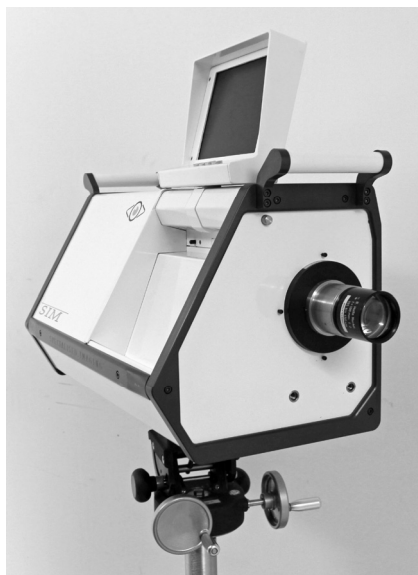
Figure 2.8 A SIM 8 framing camera with an achromatic f = 100 mm, f_{\#} = 2 B. Halle lens on a tripod, with tilt, rotation and height adjustment.
