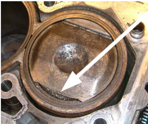
Figure 42: Damaged piston due to high PCP
