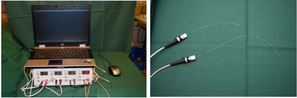
Figure3 The experimental setup using laser Doppler and filament probes.
