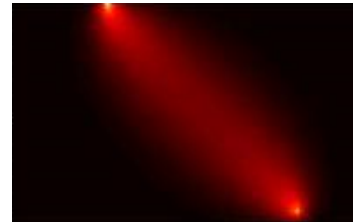
Figure 5.4. An example of the sensitivity profile between source and detector where regions with higher values will affect the measurement to a higher degree.
