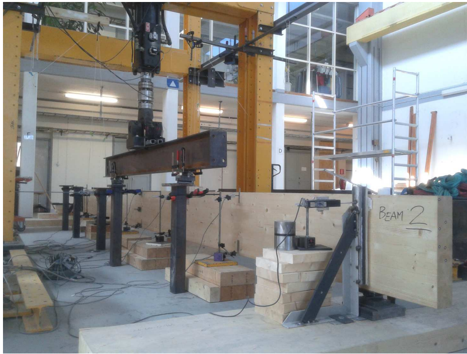
Figure 4.1: Stability testing of a simply supported and discretely braced timber beam subjected to four-point bending (Klasson et al. , 2014).
