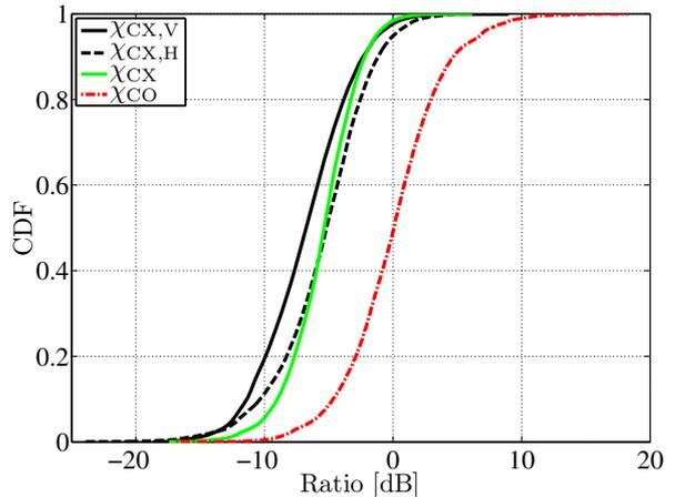
Fig. 2. The CDF of cross- and co-polarization ratios.
