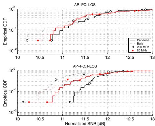
Fig. 7. The CDF of normalized SNR averaged over sub-channels (i.e. frequency diversity included) for the AP-PC ( $8 \times 4 \times 2$ , DP) scenario. The antenna subset selection is either found per sub-channel (per-tone selection) or the same subset is used for all sub-channels (bulk selection). The frequency bandwidth is 20 MHz and 200 MHz.
