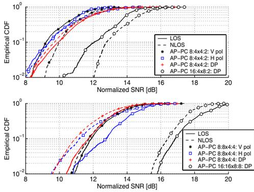
Fig. 4. Empirical CDFs of the normalized SNR for the AP-PC scenario. Two schemes are used:  $8 : 4 \times 4 : 2$  and  $16 : 4 \times 8 : 2$ , all selecting the best element subset (HS-B), with respect to SNR, on both the TX and the RX side. Results from both dual polarized (DP) and single polarized (vertical and horizontal) configurations are presented for LOS (rotation 2, 3, 6, 7) and NLOS (rotation 3, 4, 7, 8).
