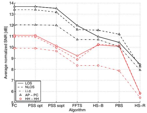
Fig. 5. The average normalized SNR for the different antenna selection schemes are presented. Both AP-PC ( $8 : 4 \times 4 : 2$  vertical polarized elements) and HH-HH ( $4 : 2 \times 4 : 2$ ) results are presented for LOS and NLOS. The same antenna selection algorithm was used at both ends. For comparison the i.i.d. channel results are presented.
