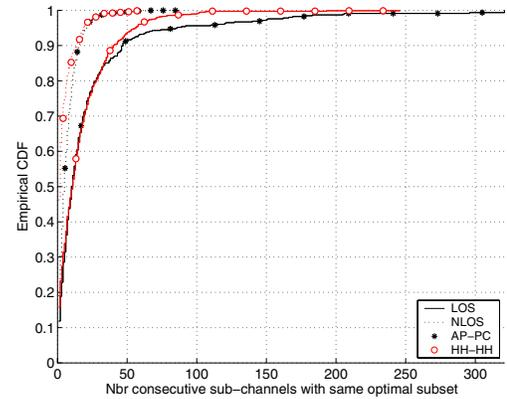
Fig. 6. CDFs of the number of consecutive sub-channels (out of the 321) that are using the same optimal subset for AP-PC ( $8 : 4 \times 4 : 2$ , DP) and HH-HH ( $4 : 2 \times 4 : 2$ ). Both LOS and NLOS scenarios are considered.
