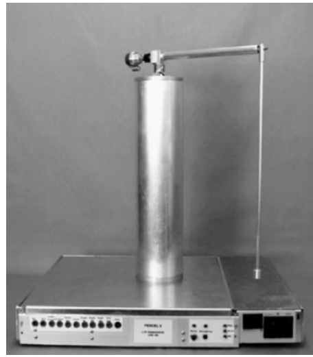
Figure 4: The Furuta pendulum.
