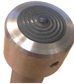
Figure 2: PCBN tool with convex shoulder
