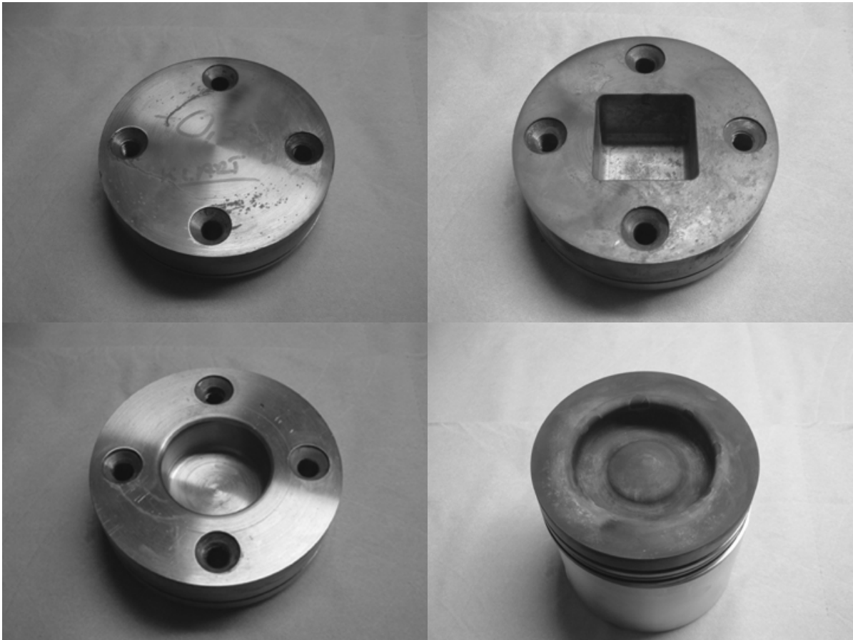
Figure 57: Pictures showing the different combustion chamber shapes tested in the metal engine experiments. Top left is the Disc, top right is the Square Bowl, down left is the Circular Bowl and down right is the standard Scania Diesel Bowl.
