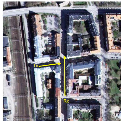
Fig. 1. Aerial image of the investigated urban crossroads scenario in the city of Lund with two vehicles moving towards the intersection at a speed of 30-40 km/h (N55° 42' 37", E13° 11' 15").
