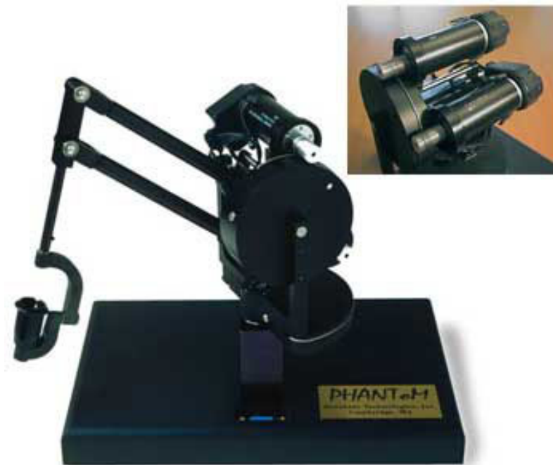
Figure 4.1 The Phantom 1.0, a haptic interface with a close-up of the motors.
