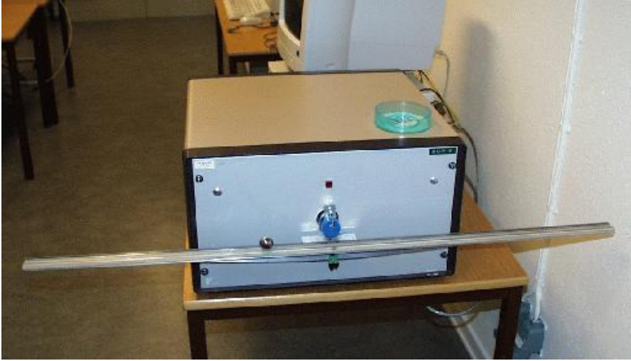
Figure 13 The ball and beam laboratory process.
