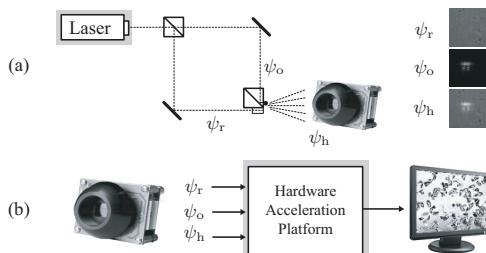
Fig. 1. (a) Holographic setup capturing the light from a laser source on a digital sensor. By blocking the reference or the object beam, totally three images are captured representing the reference  $\psi_r$ , the object  $\psi_o$ , and the hologram  $\psi_h$ . (b) The three captured images are processed by a hardware accelerator to reconstruct visible images.
