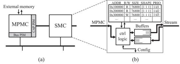
Fig. 5. (a) Stream memory controller (SMC) and multi-port memory controller (MPMC) connected to the bus system and the reconfigurable accelerator. (b) The stream memory controller (SMC) handles data transfers to and from the reconfigurable accelerator. Data is transferred in blocks and the SMC also handles memory addressing and double-buffering.
