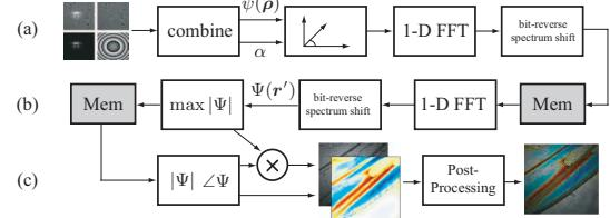
Fig. 2. Dataflow for reconstruction algorithm. Grey boxes indicate memory transfers for data reordering and white boxes indicate computation. (a) Image combine, pixel rotation, and one-dimensional FFT over rows. (b) One-dimensional FFT over columns and store maximum value. (c) Calculate amplitude or phase and scale result into pixels. Post-processing is performed on the resulting images to extract useful material properties.
