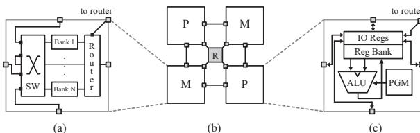
Fig. 4. (a) A memory cell (M) containing a configurable number of memory banks. (b) One tile from the reconfigurable array. (c) Example of a processing (P) containing an ALU and a microprogram.
