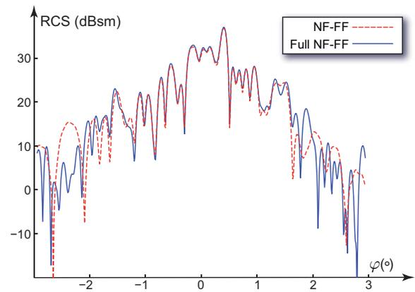
Fig. 10. RCS at  $f = 10$  GHz as a function of azimuth angle,  $\varphi$ , extracted from the complex valued data corresponding to the images in Fig. 9. Results are shown for the NF-FF and Full NF-FF methods.
