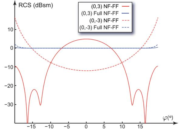
Fig. 3. RCS at  $f = 11$  GHz as a function of azimuth angle,  $\varphi$ , extracted from the complex valued data corresponding to the images in Fig. 2 for the point targets at  $(0, -3)$  and  $(0, 3)$ . Results are shown for the NF-FF and the Full NF-FF method
