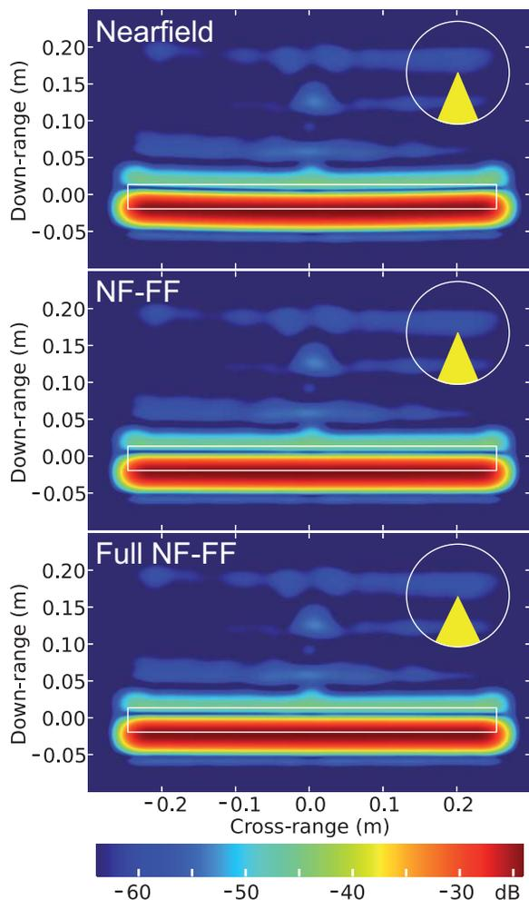
Fig. 4. The images show a measurement of a cylinder positioned at the turntable center, the origin, with  $r_0 = 7.6$  m. The top image is processed assuming infinite distance, the middle image using the NF-FF method and the bottom image the Full NF-FF method. The angular interval is at  $0^\circ$ . A Hanning window is used for all images. The filled circle sectors show the part of the angle interval that are used for the images.
