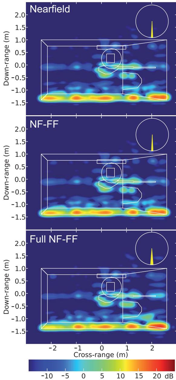
Fig. 9. The images show a measurement of the right, wheeled side of the STANDCAM target positioned at the turntable center, the origin, with  $r_0 = 101$  m. The top image is processed assuming infinite distance, the middle image using the NF-FF method and the bottom image the Full NF-FF method. The angular interval is centered at  $0^\circ$ . A Hanning window is used for all images. The filled circle sectors show the part of the angle interval that are used for the images.
