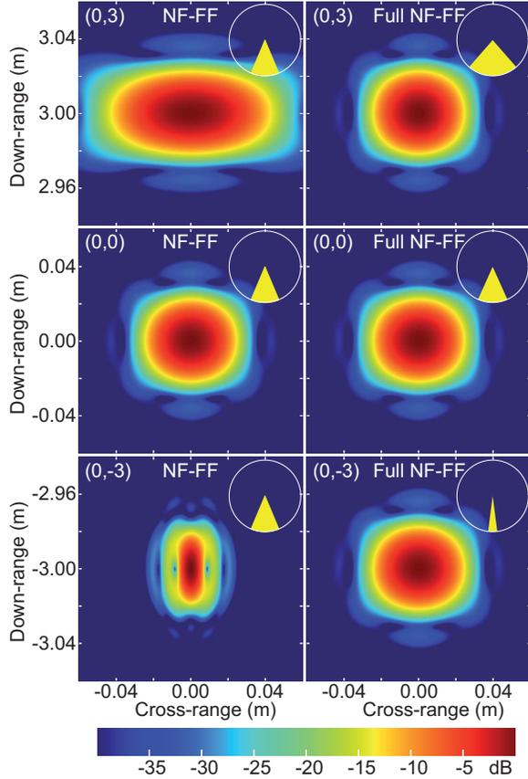
Fig. 2. The images show isotropic point targets positioned at  $(0, -3)$ ,  $(0, 0)$  and  $(0, 3)$  with  $r_0 = 4$  m. The left and right columns are processed using the NF-FF and Full NF-FF methods, respectively. A Hanning window is used. The filled circle sectors show the part of the angle interval that are used for the images.
