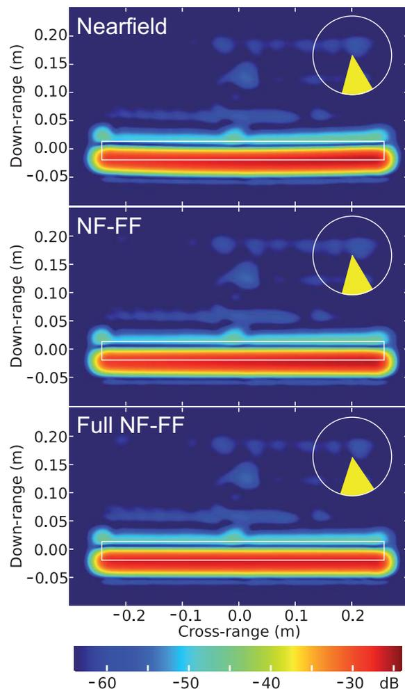
Fig. 5. The images show a measurement of a cylinder positioned at the turntable center, the origin, with  $r_0 = 7.6$  m. The top image is processed assuming infinite distance, the middle image using the NF-FF method and the bottom image the Full NF-FF method. The angular interval is centered at  $+8^\circ$ . A Hanning window is used for all images. The filled circle sectors show the part of the angle interval that are used for the images.
