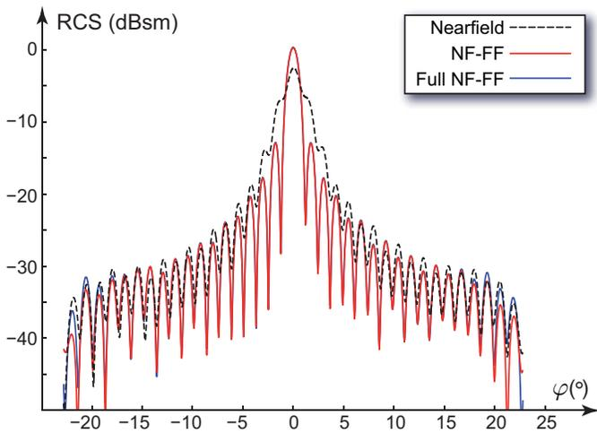
Fig. 7. RCS at  $f = 11$  GHz as a function of azimuth angle,  $\varphi$  extracted from the complex valued data corresponding to the images in Fig. 4. Results are shown assuming infinite distance to the target, using the NF-FF method and the Full NF-FF method.
