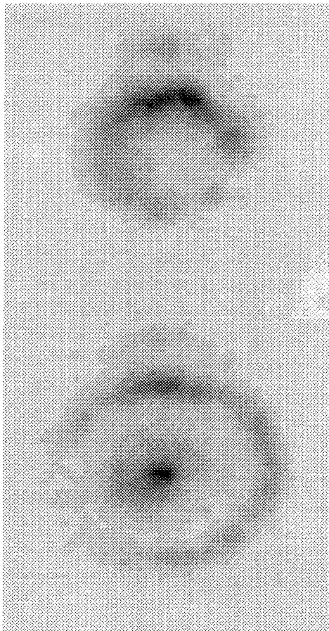
Fig. A3. Examples of two far-field spatial intensity distributions of the 13th harmonic. The different images represent different settings of the Babinet compensator, and illustrate the ability to control the spatial mode of high-order harmonics.
