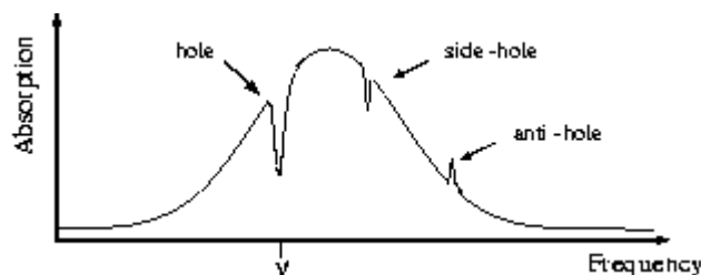
Figure 5: The absorption profile as probed after a hole burning experiment
