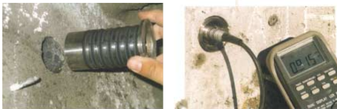
Figure 7: Mounting of proprietary corrosion sensors in existing quays. The picture to the right shows the sensor, a temporary micro-amp meter and the small titanium pin as cathode placed just above the instrument. The system is a further development from the system in Schiessl and Raupach 1992.
