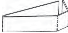
Fig. 2 Representation of a laser cut and bent Voronoi cell
