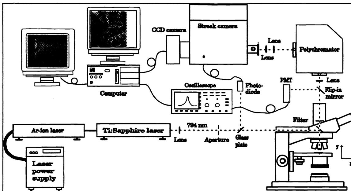
Fig. 1: Experimental set-up.
