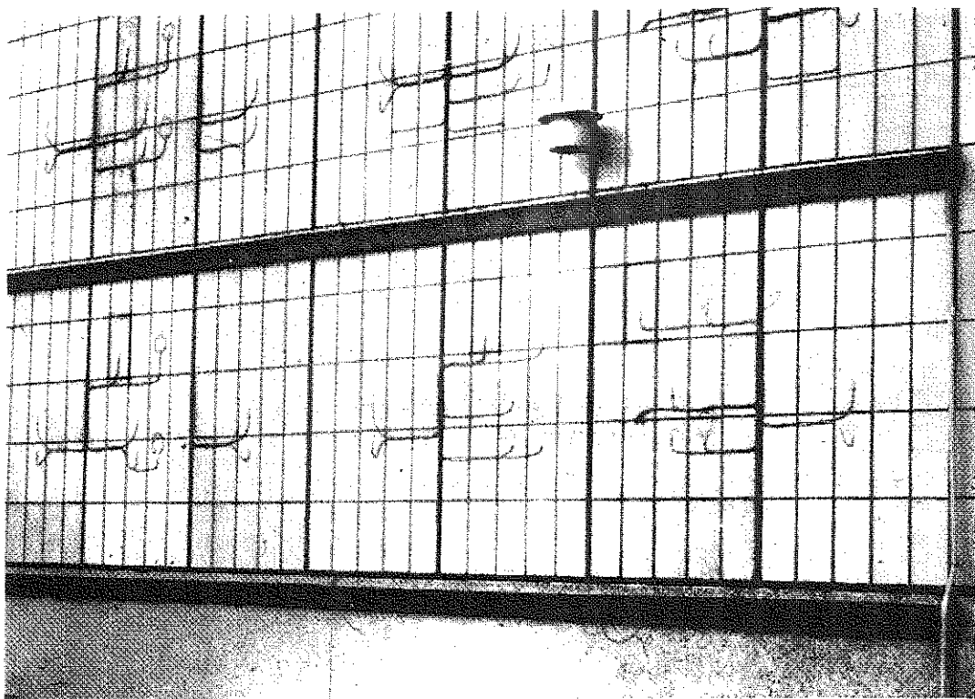
Fig. 40.5. Completed wall with strain-gauged tiles and cables
