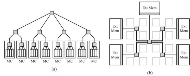
**Figure 4. (a) Hierarchical connection of routers to memory cells, (b) On-chip scratch pads or external memory connected to routers. The designer specifies where to connect memory controllers for external memory.**
