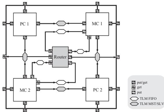
**Figure 7. A basic cell containing two processing cells, two memory cells and a router for global communication. All modules in the system communicate through master-slave or FIFO channels. Master-slave channels contain two FIFO channels to support bidirectional communication.**
