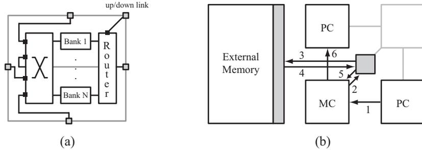
**Figure 2. (a) Internal building blocks in the memory cell, consisting of a port switch and four memory banks. Each memory bank has a unique ID for routing data over the network. (b) Two memory cells using the external memory interface to transparently emulate a larger buffer.**
