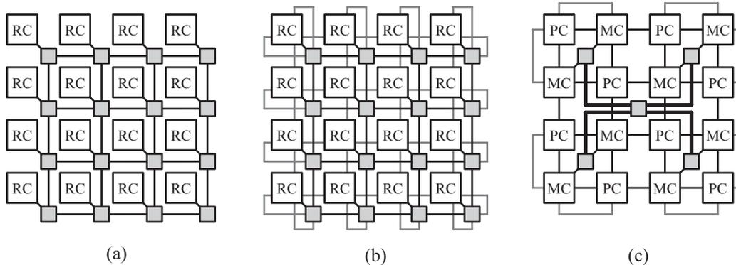
**Figure 1. (a) 2D mesh with resource cells, (b) Torus, (c) Proposed architecture with nearest neighbor and hierarchical communication. In this example, four basic cells are connected together using dedicated wires for local communication and five network routers for global communication.**
