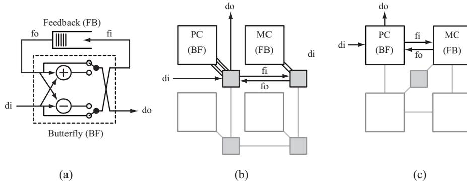
**Figure 3. (a) Butterfly and delay feedback memory, (b) Mapped to a mesh architecture, the communication bandwidth limits the performance and resulting in a utilization of 50%, (c) Mapped to the proposed architecture, the communication and processing is balanced resulting in 100% utilization.**
