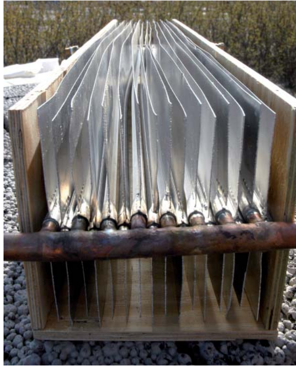
Figure 4.12 The heat exchanger. The fin pipes are not straight, resulting in a wavy path for the air through the exchanger. Photo Hans Follin.
