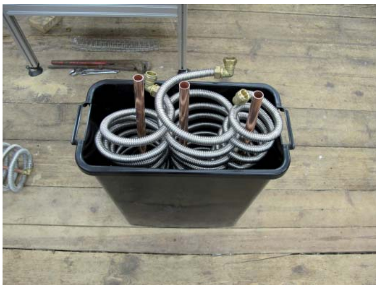
Figure 5.1 The heat exchangers inside the waste water tanks.
