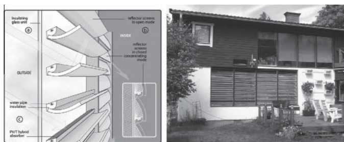
Fig. 1. Left; the solar window with water cooled PV cells, tiltable reflectors and anti-reflection treated glazing. Right; the solar window in Solgårdén.
