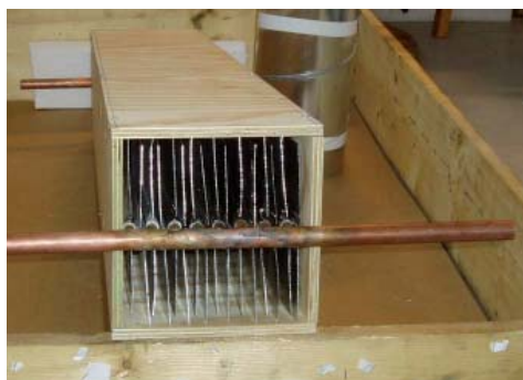
Figure 4. The fin pipes soldered to the manifold in the heat exchanger.
