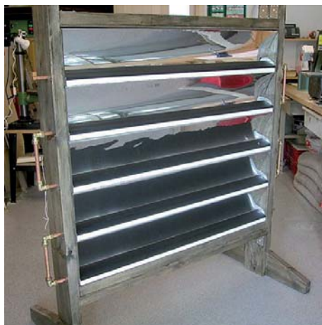
Figure 3.4 The prototype solar window with five absorbers and five reflectors. The uppermost absorber is laminated with PV cells.
